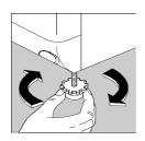
Make the washing machine level by adjusting the leveling screw that is too short. Unscrew the stand and locking collar assembly (lift the washing machine if necessary).
